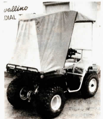
Cab rolls up and stores in a roll in front of handlebars.
