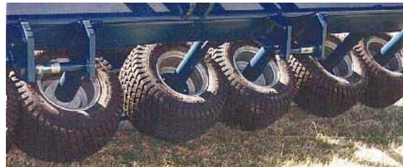
A gang of heavy duty 8-in. turf tires mount on drive shafts up front and are chain-driven off a ground-driven gearbox on the machine’s left side.
