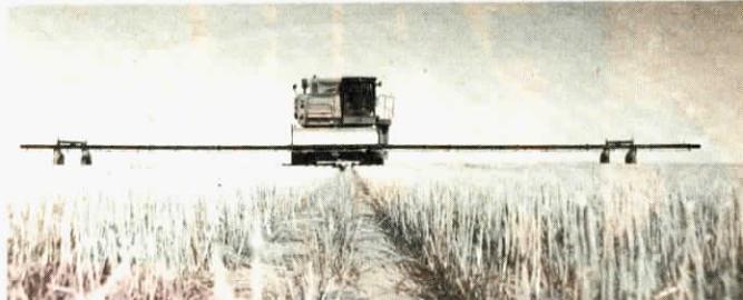
The 80-ft. booms are made of 6-in. dia. steel tubing supported at each end by a pair of castor wheels.
