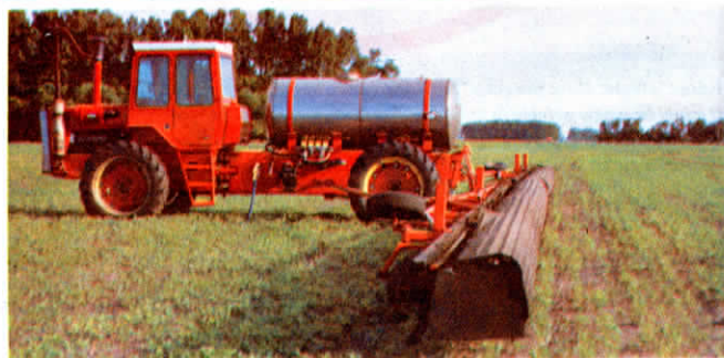
The Goodykes extended the rear frame of the tractor 5 ft., at the same time lengthening the driveshaft. Shields on spray boom prevent spray drift.
