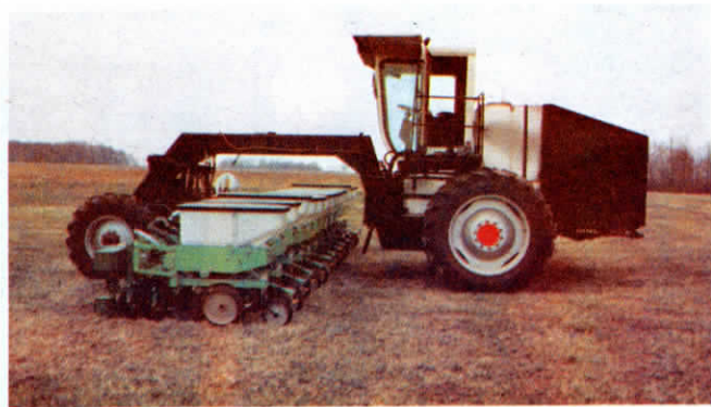
Buening uses a sled to slide implements underneath the bridge hitch to mount on the front 3-pt.
