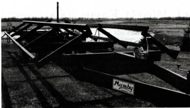
Five or six turns of hand crank dump both bale cradles.
