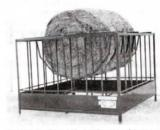
pended basket with feeder panels around the outside. Because cattle eat at an accessible height, they don't back out while feeding. A wood floor can be installed by the purchaser under the bale so dropped hay will fall on a dry surface, giving cattle a second chance to clean it up.
