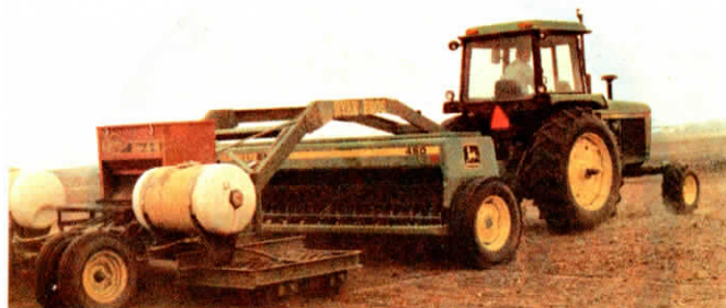
The culti-mulcher was originally equipped with two rollers spaced 7 ft. apart with field cultivator shanks in the middle. Ryan removed the shanks and hitch, then moved the rollers in so they're 8 in. apart. Alfalfa seed is delivered between the rollers.
