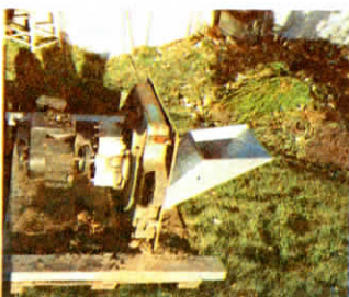
Hunt mounted the mower on its side and fitted an intake hopper to the bottom.
