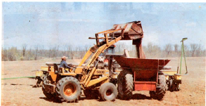
Steinacker fills the cart with the bucket on his Case tractor. He closed in the open front of the bucket, installing a 1-ft. trap door at the bottom that opens by pulling a rope.
