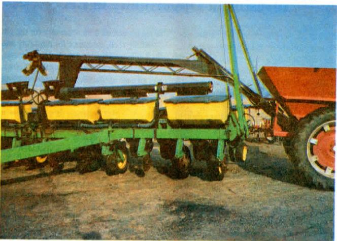
A pair of augers mount on the bridge hitch which runs from the cart up to the planter. Photo shows planter "jackknifed" back under the hitch.
