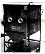
"Inside the hopper I installed a wire mesh grate to set parts on. Any size mesh will work as long as sand can fall through to the bottom to be recycled.
