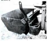
This is a good way to carry rocks in from the field without handling them twice. I hung a trip bucket on the front of my IH tractor. I throw rocks and other debris into it while in the field and simply pull the lever to dump at a rockpile. The spring-loaded bucket came from a manure loader. It's got a slip-on mount so it'll go on or off the tractor in seconds. (Roy Davis, Clemons, lowa 50051 (ph 515 477-8580)
