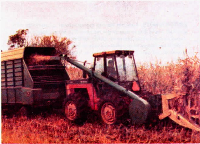
Photo shows pull-type Deere 3800 chopper carried on front 3-pt. of Versatile's Bi-Directional 276.
