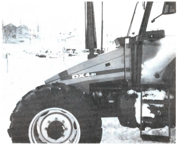
Deutz tractors are the easiest to modify because they have air-cooled engines, eliminating the need to lower the radiator.
