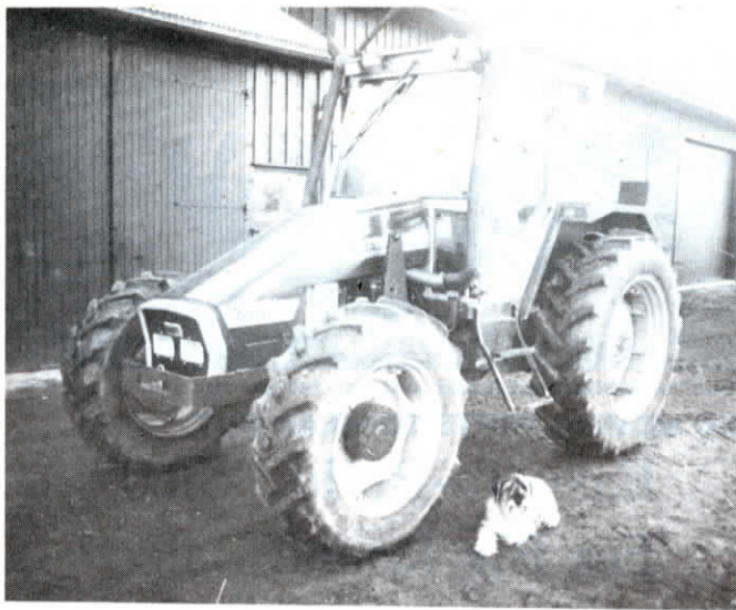
"Plastic surgery" to the front engine cowling of loader-size tractors results in better visibility by moving the radiator, battery, and air cleaner away from front of engine.
