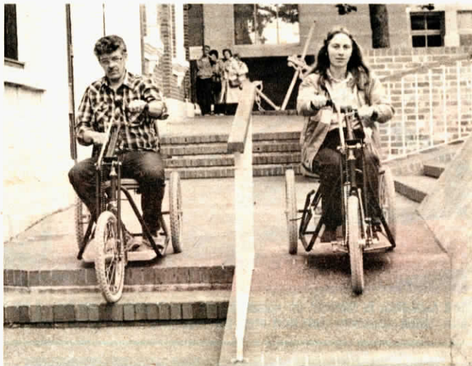
Hand-pedaled knobby bicycle wheels travel easily over obstacles.
