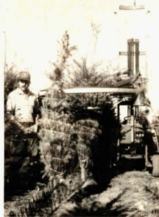
Baling ring wraps twine tightly about standing trees.
