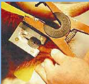
Add-on attachment uses V-shaped blade to slice off old tags.
