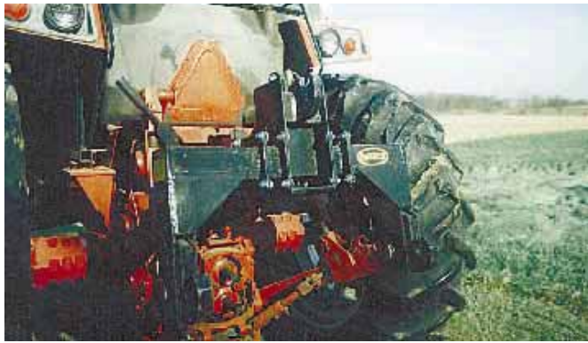
Width adjusts by adding, removing spacers. Height adjusts by moving center hitch point up, down.
