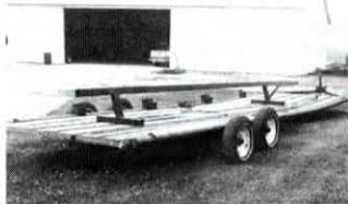
We have a few narrow bridges to cross when traveling between fields with our combine and we can't get across with the header in place. I already had this low implement trailer that was not used during harvest so I decided to adapt it to carry a header using a few pieces of square tubing. Works very well and is easy to remove when harvest is over. (Curt Melner, Colfax, Ill. 61728 ph 309 723-6225)
