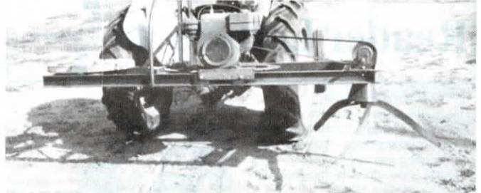
I built this "weed whopper" to keep several miles of electric fence free of weeds. I mounted a straw spreader from a Deere 95 combine on the end of a heavy steel frame that runs across the back of the tractor, mounted on the 3-pt. Three thick strips of rubber hang from the bottom of the straw spreader, which is belt-driven by a 10-hp. Wisconsin gas engine. A tractor weight lays
