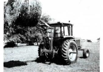
My "Hydra Stinger" rear-mounted bale loader sells for about half the price of a front-end loader and makes bales easier to handle since more of the weight is on the rear of the tractor. The loader is automatically self-leveling and mounts and dismounts quickly, as needed. Can handle round and square bales, stacking bales 3-high in the barn or 2-high on a truck or trailer. (Byron Coats, Hydra Stinger, P.O. Box 531, Tuttle, Okla. 73089 ph 405 381-4144)
