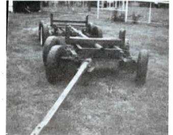
I built this 8-wheel wagon with 4 steerable wheels up front back in the early 1970's. When I first built it, the wagon had 2 axles in back and a single axle up front. To even out the load, I decided to add a second axle up front that would oscillate in both directions. To do that, I needed to design a new steering linkage.
