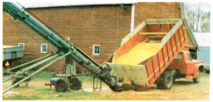
Both augers are powered by electric motors, one mounted on a portable 2-wheel cart and the other mounted directly on top of one auger.
