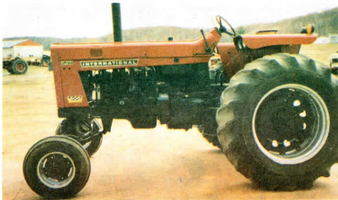
Link repowered this IH 806 gas tractor with the same Cummins diesel engine used in new Case-IH Maxxum tractors.
