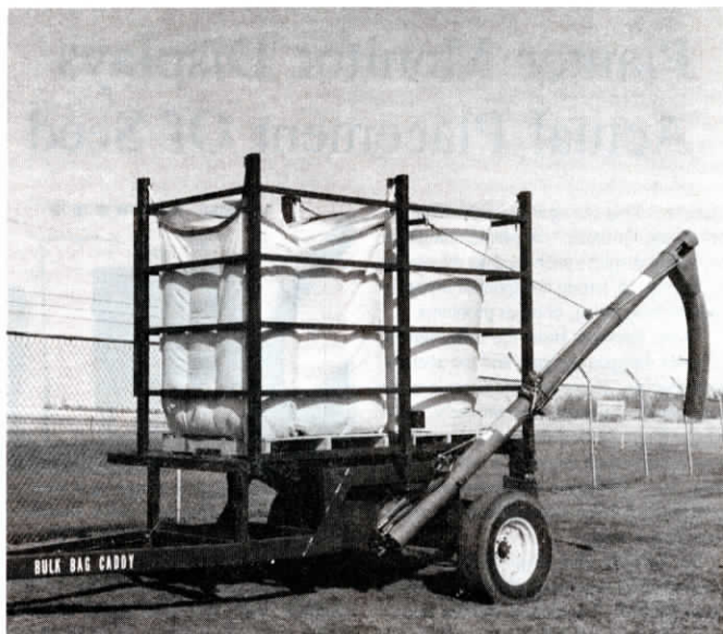
Caddy is equipped with pair of "cages" over steel platform. Bags feed into hopper-mounted auger.
