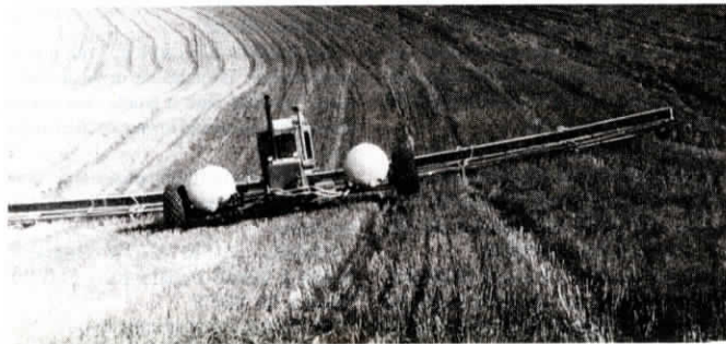
A pair of 500-gal. spray tanks mount on flexed frames that attach to each side of Caterpillar. Frame is hinged so tires can flex up or down.
