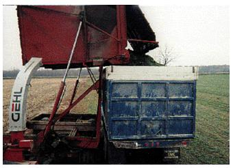
Cover of wagon opens automatically when wagon lifts for dumping. Hydraulic-driven apron chain on side of wagon helps dump into trucks.
