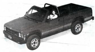
Top folds down behind cab or can be removed to leave pickup bed free.
