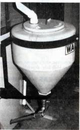
Add-on 15-gal. hopper adds liquid feed supplements evenly to feed, virtually eliminating dust as feed comes out of grinder-mixer.
