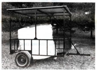
Winch-powered bale spear holds bale upright inside feeder for feedout or transport.
