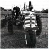
Variable speed hydraulic controls mount on a rear fender so speed can be controlled from the ground.
