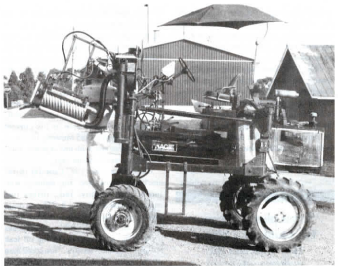
Self-propelled "corn pollen harvester" was made by modifying commercial 4-row "high-boy" corn detasseling machine.
