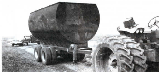
Cylinder-shaped wagon is 8 ft. in dia. and 16 ft. long. It holds 600 bu. of corn.
