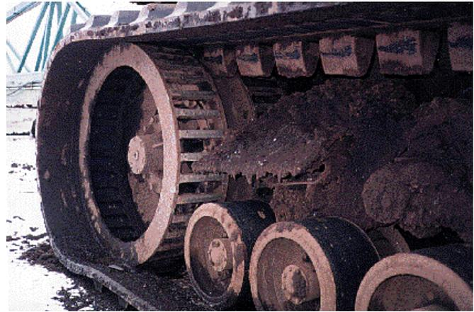
Steel bars don't wear as fast as rubber and are narrower so mud cleans out quicker.
