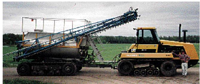
Boom hydraulically folds forward for transport. Platform on top of tank makes filling easy.
