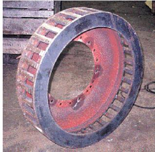
Horodynsky welded thirtysix 1 1/4-in. wide steel bars onto outside part of original driver wheel rim. Bars extend 1/8 in. beyond rim to provide a better grip.
