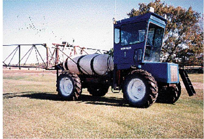
Roy used the frame, axles, engine, and transmission from a Dodge 1-ton truck, cab from a New Holland combine, and flotation tires from a Massey Ferguson combine.
