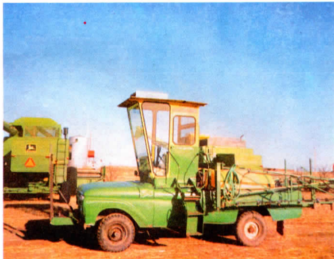
Bruckner mounted old Deere combine cab on 1966 Ford 3/4-ton 4-WD pickup. A 300-gal. spray tank and 48-ft. boom mount in back of pickup.
