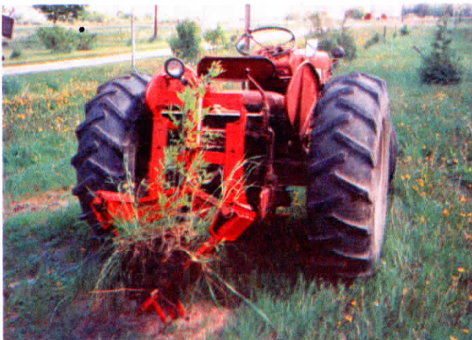
Tree fork is designed to transplant trees up to 1 in. in diameter.
