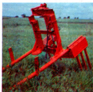
Unit has two digging forks, each equipped with three 1-in. sq. steel tines.
