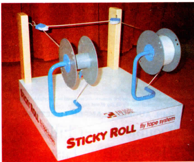
System consists of two crank-up reels that mount anywhere in barn. As sticky tape fills up with flies, it's cranked up onto empty reel.
