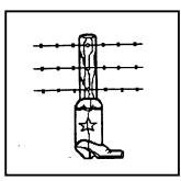
Plastic "boot" slips over bottom of post and has drain holes in the bottom. (Boot doesn't really look like a cowboy boot!)
