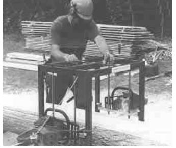
Sawmill's 22-in. wide carriage is equipped with a single chain saw-type cutterbar powered by a chainsaw power unit mounted on either end.
