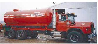
Mueller mounted a 4,000-gal. liquid manure tank on a used Mack tandem axle truck. Hydraulic-powered shuttle arm hooks onto a steel subframe bolted on under tank.
