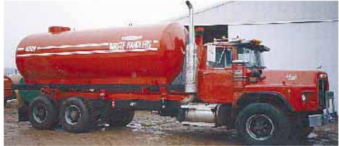
Mueller mounted a 4,000-gal. liquid manure tank on a used Mack tandem axle truck. Hydraulic-powered shuttle arm hooks onto a steel subframe bolted on under tank.
