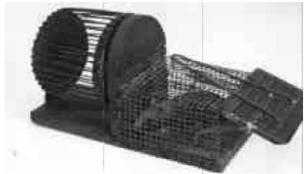
This trap was called the "Wheel of Death". When mouse goes after bait a spring-loaded door snaps shut behind him and he's caught inside a square wire cage. He then goes through a hole and is trapped inside a cylinder-shaped cage that spins around freely. He can't get back out and runs himself to death.
