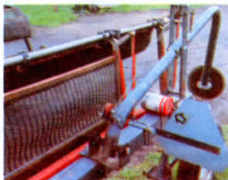
Cameras are encased in plastic peanut butter jars.
