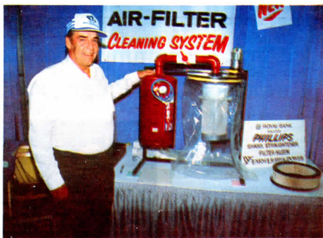
Phillips' kit consists of small air tank with pipe out the top that hooks up to dirty filter, which is enclosed in a clear plastic bag.
