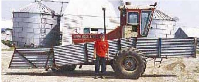
Chute is welded to right side of combine in place of detachable harvesting unit.
