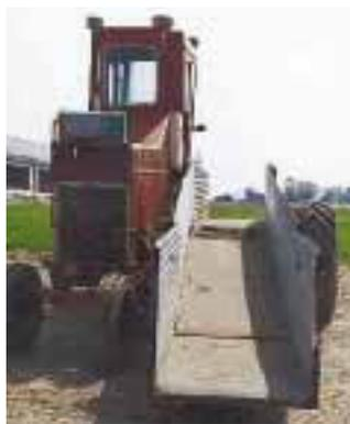
Rear view of loading chute shows rough concrete floor made in 3 hinged sections.
