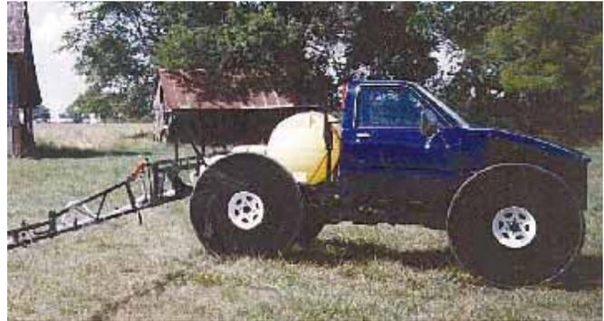
Hall turned a 1982 Chevy Luv pickup into narrow-wheel sprayer with steel wheels covered by a band of 1 1/2-in. thick rubber.
