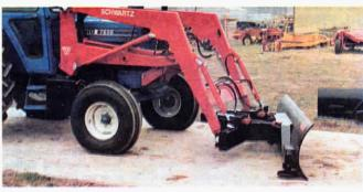
Completely hydraulic, the new blade tilts in either direction, and up and down at the ends for laying a grade.
