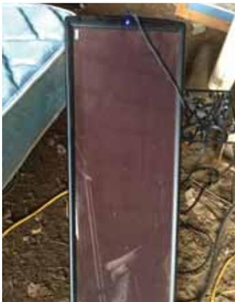
Danczyk uses a 14 by 25-in. solar panel to charge the three 36-volt batteries that power his e-trike.
