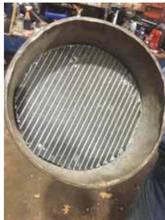
An old radiator core can be used as a pre-cleaner in front of an existing radiator.
