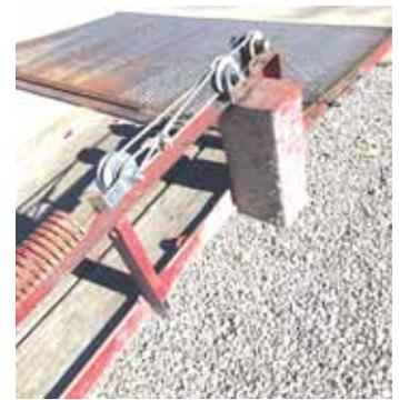
Vandeventer used a heavy spring to make his own fold-down ramp lift assist.
