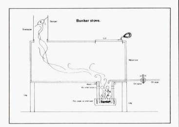
In this home-built waste oil heater, the oil is dripped into a pot and, being vaporized, it burns with a yellow-bluish flame. The system operates with good access to air so the lean mixture makes the oil burn clean.
