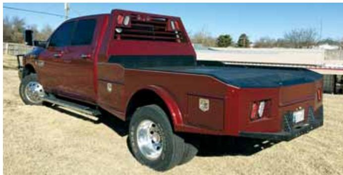
**Schmidt's standard flatbed includes a steel floor, custom headache rack, 4 under-the-bed toolboxes, LED lights in the window, and a rear bumper.**
