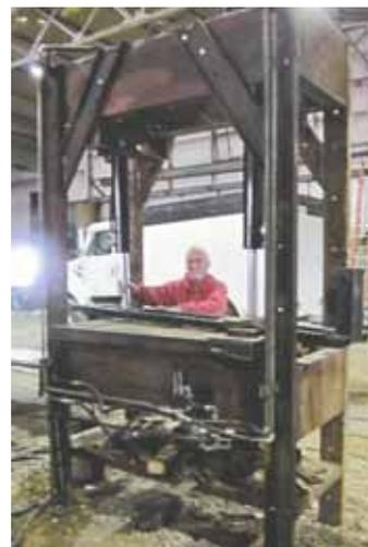
**The big cylinders on Wilson's giant press move back and forth freely to adjust to the job.**
