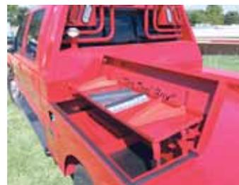
**Schmidt can also fit flatbeds with low-profile toolboxes that open on the bed of the truck but don't interfere with goosenecks.**
