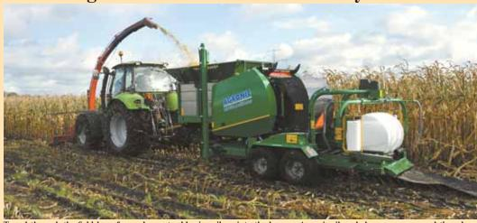
Towed through the field by a forage harvester blowing silage into the hopper, Agronic silage baler compresses and then drops plastic-wrapped bales out the back.
