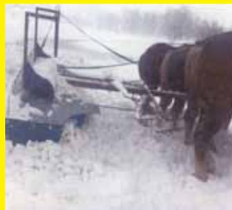
Thank you for your article a year ago on our dumping snow blade made out of a curved Harvester silo panel. It's designed to be pulled by a 2 or 4-horse hitch and we've used it since 2010. Last spring we redesigned the tongue latching and unlatching system to improve operating efficiency. It lets anyone who doesn't have a skid steer or tractor snowblower clear a driveway easily using horses. (**Jesse Fisher, 347 School Lane Rd., Gap, Penn. 17527 ph 717 442-8958**)
