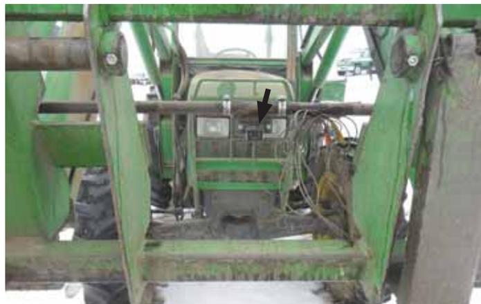
**Back-up camera mounts on loader tractor frame behind the forks. "It's especially helpful for seeing anything down low on the ground where my view normally is blocked," says Ted Lacy.**
