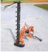
Hydraulic drive provides cutting action no matter what angle the bar is at, from horizontal to vertical.
