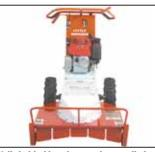
Walk-behind brush cutter has small plates on front that swing to keep rocks and debris from shooting out.
