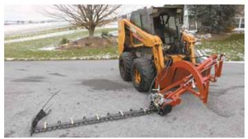
Front-mount sicklebar mower makes it easy to see what you're cutting. "Works great for cutting weeds and grass along pond edges and fences," says the company.
