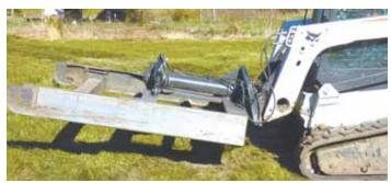
He can tilt the blade up and down and left or right, thanks to a unique mount that uses an old sheeps foot roller tongue and bushings.
