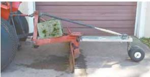
2-wheeled, triangleshaped attachment makes Timothy Hoopman's 3-pt. mounted blade work more like a road grader.
