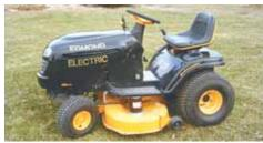
Brian Edmond converted this gas-powered lawn tractor to electric. It has 3 motors: one for the drive system, and 2 smaller ones mounted directly to the mower blades.
