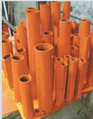
**Gene Boehler, Farmersville, Ill.:** "I needed a better way to store tools while at the same time keeping them readily accessible, so I put several short pieces of steel pipe and tubing to good use. They're in various sizes and measure from 6 to 12 in. long. I placed the pipes and tubing in rows about 1 1/2 in. apart. Then I welded them to an 18 by 20-in. base made from 1/8-in. thick steel plate that forms a base, then painted everything bright orange.
