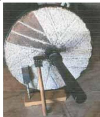
Wayne Beggs welded a Tampo rock pick tip on a Snap-On air chisel, cutting off the chisel. The result is a small jack hammer that makes it easier to dress millstones when they get dull. He also use a facing hammer.
