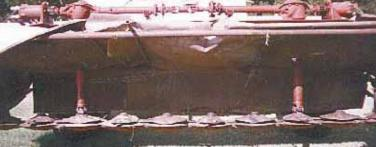
"It lets me mow thick hay at 10 mph," Tom Cathey, Covington, Tex., who built a hydraulic-driven rotary cutterhead by mounting two auto rear ends on top of head and running drive shafts down to U-joints mounted on top of cutting discs. See story on page 3.
