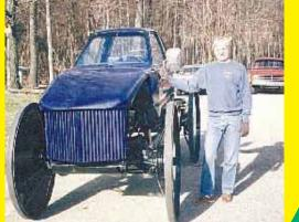
Narrow 2 1/2-in. wide wheels and a cut-down cab make this crop sprayer unique. Larry Hall, Clarkston, Mich., cut 20 in. out of the center of the cab and made a new hood in order to provide enough room for the 4-ft. tall, narrow steel wheels to turn. The narrow wheels let him spray solid-seeded beans without doing damage. See story on page 2.
