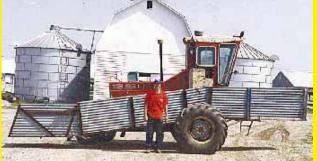
To avoid building a loading chute at each of his eight different finishing buildings, Illinois hog producer Allan Weitekamp built a portable loading chute by mounting a hydraulic-powered chute on the side of his New Idea Uni-Harvester combine. See story on page 2.
