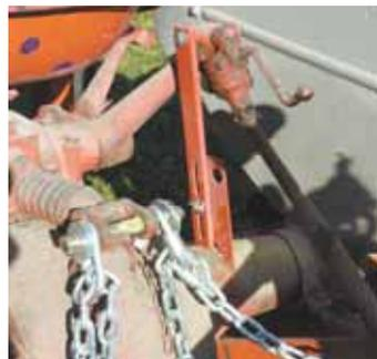
the pto is not engaged. I previously added limiting chains to prevent attachments from falling too far when in use. However, that can still be lower than I want when transporting them. The lock resolves the issue.
