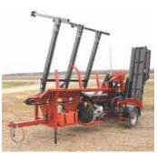
Watson Scott, Middlebury, Ct.: "I like my 2014 Brute Force 18-24 HD firewood processor (www.bruteforcemfg.com; ph 715 245-2144). This machine is ideal for maximum wood production and has features that other, more expensive brands don't have. It's easy to use and can handle 20-in. dia. logs up to 16 ft. long."
