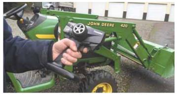
Brian Laine used mostly off-the-shelf parts to convert his Deere 4210 to a remotecontrolled tractor. A standard RC controller is used to operate the tractor.
