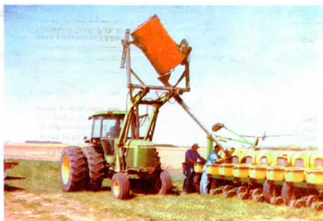
Tank mounts in frame on Deere loader and is hydraulically rotated to mix seed and inoculant. Treated seed is then gravity fed down pipe and into planter boxes.
