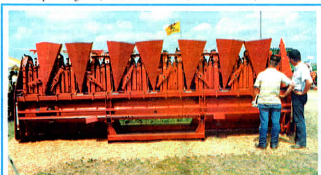
Knives mount under snap rolls and cleanly chop stalks into 4 to 5-in. pieces.
