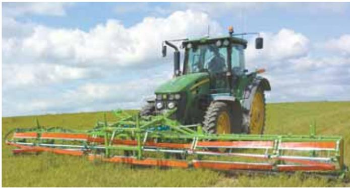
Last year organic farmer Colin Tanner used this Swedish-built, mechanical weeder called CombCut to clean up his small grain fields. The folding toolbar can be mounted ahead of or behind the tractor.
