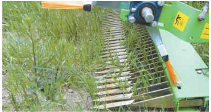
Machine combs through flexible stems of wheat and other small grains, cutting away broadleaf and other thick-stemmed weeds.
