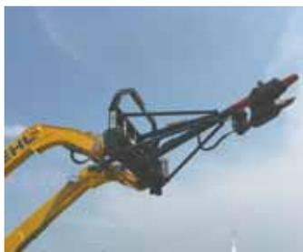
Telescoping boom hydraulically extends Precision Tele-Clipper head from 7 ft. 3 in. to 10 ft. 3 in.
