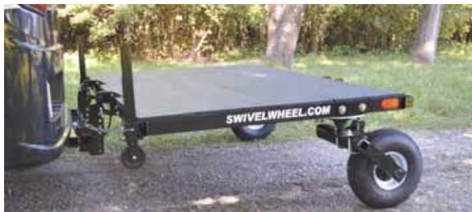
SwivelWheel trailer lets you haul motorcycles and ATV's without the hassle of backing up a jackknifing trailer.
