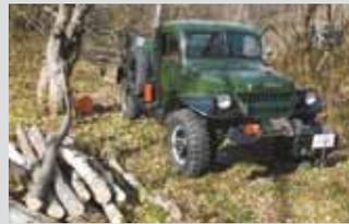
**Clint Dixon says his 1947 Dodge WDX 4-WD, 1-ton Power Wagon is a "best buy." It has both front and rear pto and can be equipped with a hydraulic lift. Dixon pulls a 3-bottom plow and runs several pto-driven attachments, including a buzz saw and a wood splitter.**
