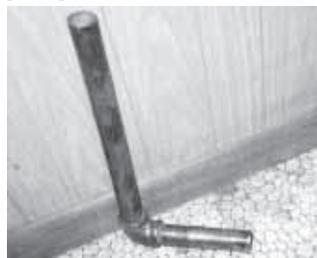
I made one using his directions and it’s the handiest fencing tool I have. It’s made from two 1-in. pieces of pipe connected by a 90 degree elbow. The handle, is 16 in. long and the other is 8 in. long. A 5/16-in. dia. hole is drilled through the 8-in. piece, 2 in. out from the elbow.
