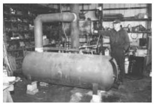
Hemingway built the wood furnace out of a 250-gal. anhydrous tank.
