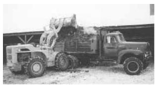
Used Farmhand manure spreader mounts on 1960's all-wheel-drive International tandem axle truck. Box is equipped with two rear beaters.
